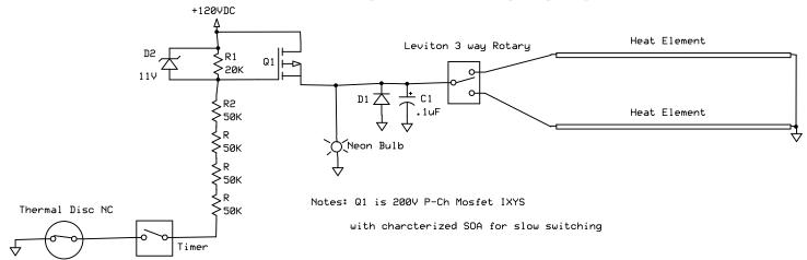
Diode D1 and Cap C1 to supress inductive kickback
